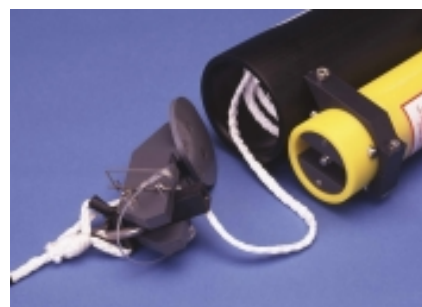
Rope deployment following a secure 'release' command from the surface.
